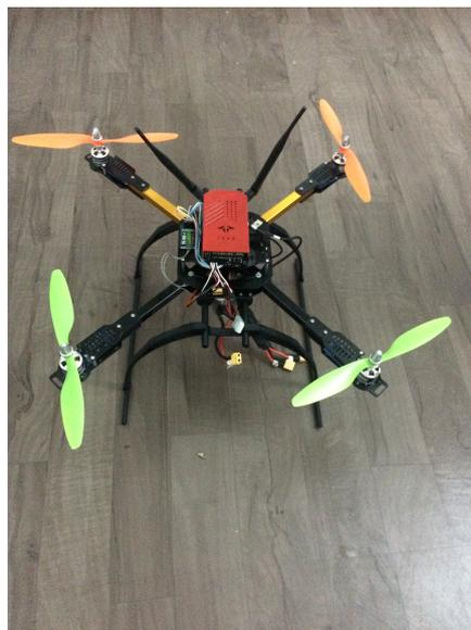
(b) With propellers and landing gear
