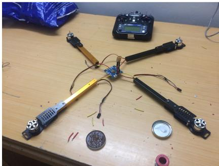
(d) Connection of the motors, ESC and distribution board
